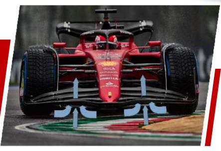
The downforce on a Formula One car is achieved by the two wings on the front and the back of the car. These wings push the air around the car in a way that reduces air resistance but also creates downforce to give the car a good grip on the road.
